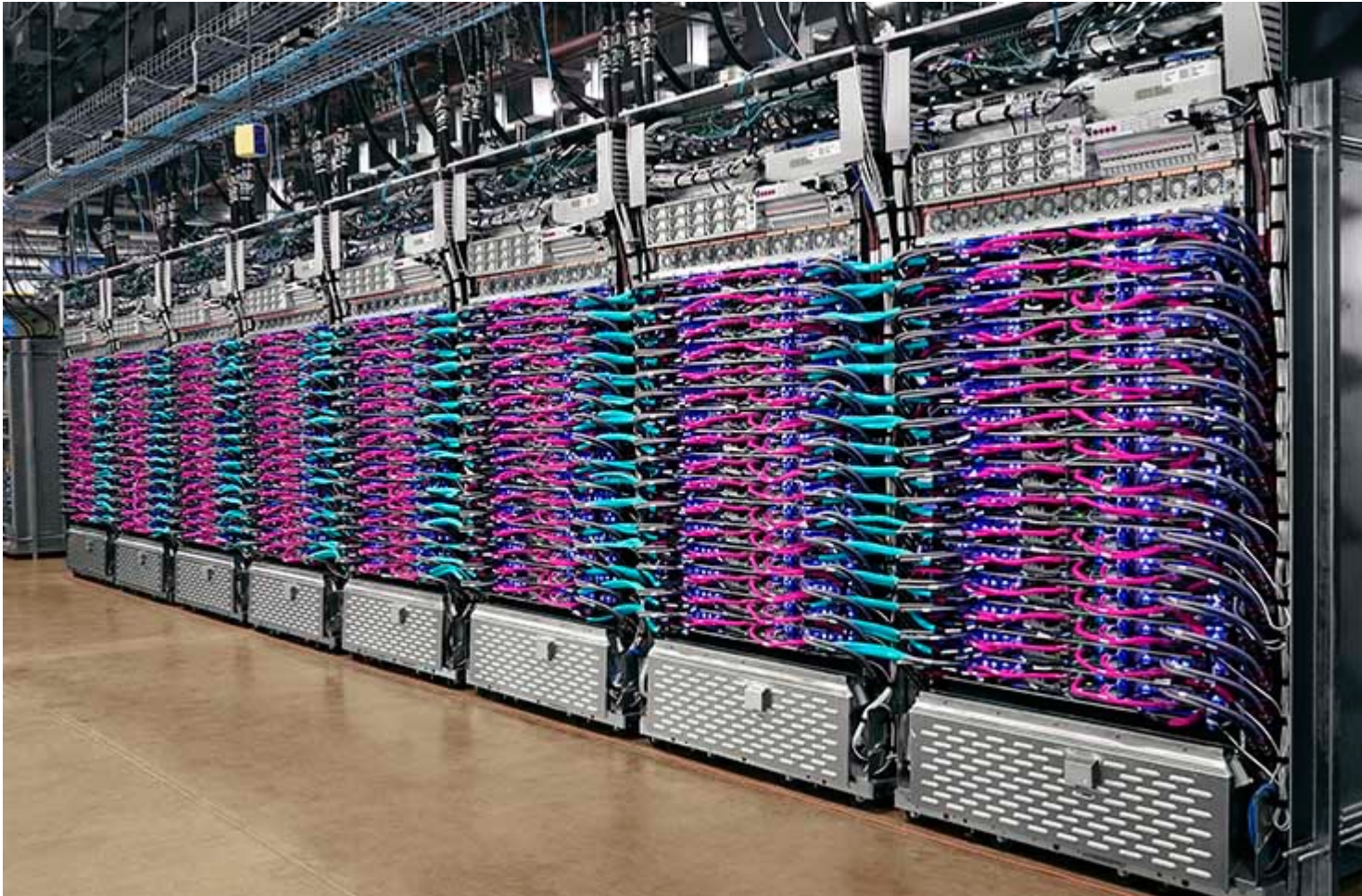
An eight-rack pod of Google's liquid-cooled TPU version 3 servers for artificial intelligence workloads. (Image: Google)
